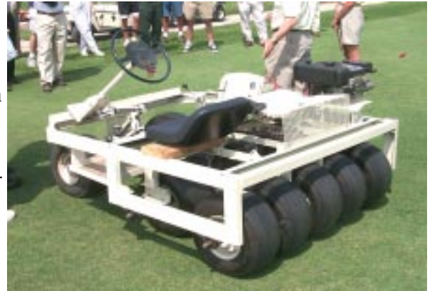
Apparatus built by Nebraska turfgrass science team members to simulate golf cart traffic. The unit delivers consistent and uniform traffic patterns and is used on many NTEP trials as well as other research projects.
